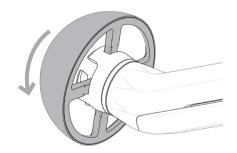
To detach, twist reamer anticlockwise and remove reamer
