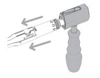
Ensure the handle securely locks into position by pushing it towards the Angled Body until you hear an audible click.
