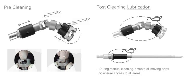
• Post cleaning, apply lubricant to all joint areas as highlighted, to extend longevity of your device.
