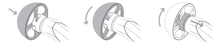
Note that if the drill is not attached you may need to hold the protruding end of the Drive Shaft to prevent rotation of the coupling head.
